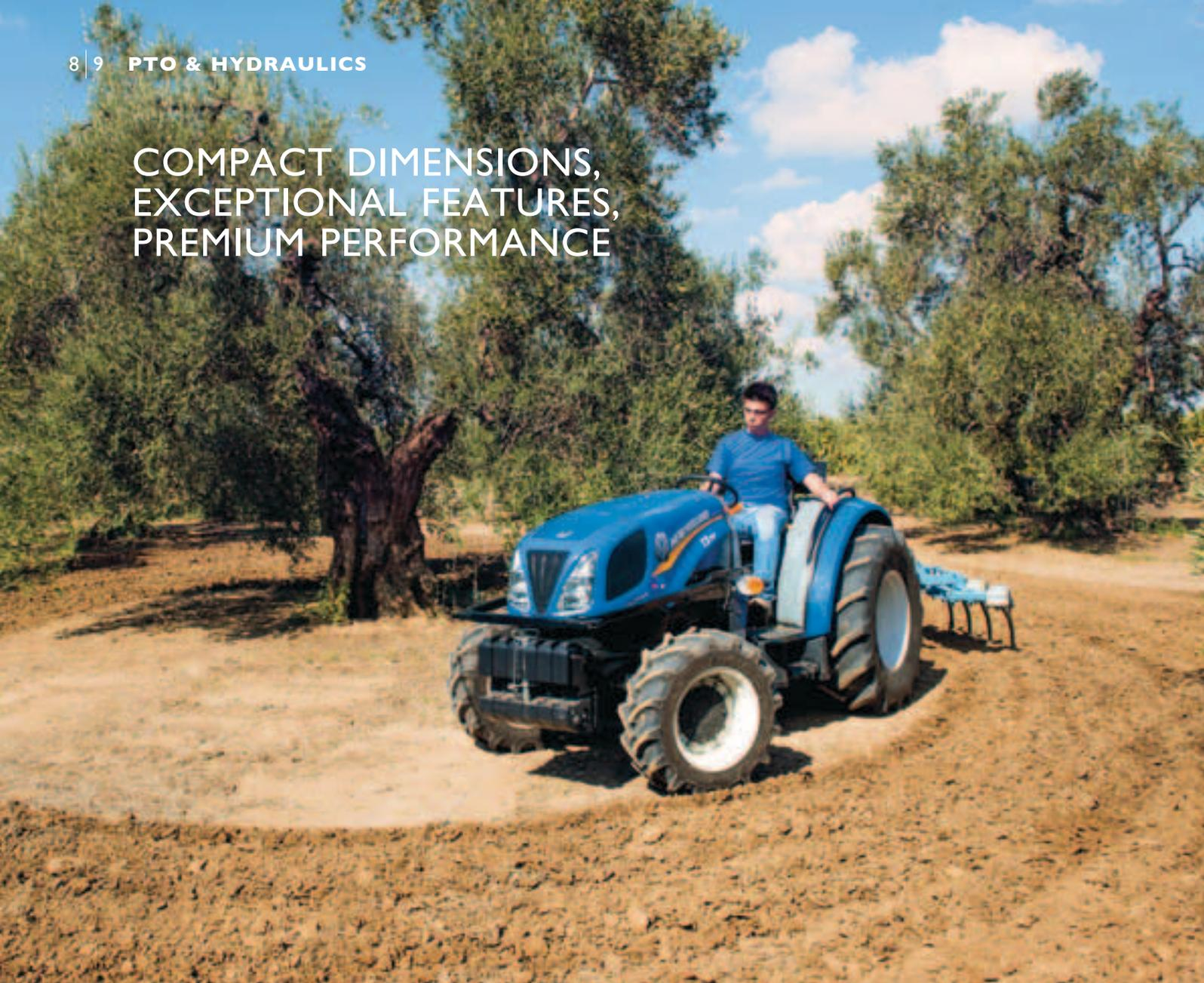
Lighter and shorter than the award winning specialised T4000F/N/V series tractors, the new T3F machines are on a par with their “big brothers” in terms of features. Hydraulic rear hitch with two external hydraulic rams, lift capacity of up to 2277kg and Lift-O-Matic™ system supplied as standard. Two separate pumps for the hydraulic circuit and steering. Up to 3 remote valves. Servo-assisted PTO with up to 3 speeds.
