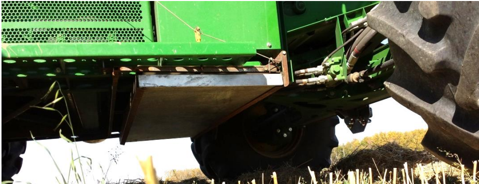
Figure 3-4. Loss pan dropper installed on a JD combine.
