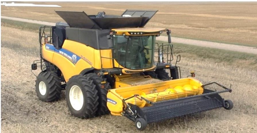
Figure 3-1. New Holland CR9.90 Elevation combine with belt pickup header.
