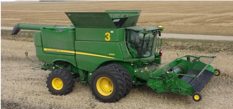
Figure 3-2. JD S690 combine with 615P belt pickup header.
