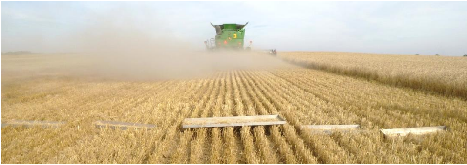
Figure 3-6. Loss pan layout for chopper and spreaders engaged loss collection.
