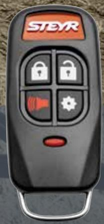
STEYR has integrated useful functions into the key fob. Apart from locking and unlocking the cab with the push of a button, the new key fob also protects against unauthorized access and theft, since the tractor won't start without a recognized key.
