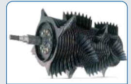
Crop-Cutter™ System + Hydraulic Reverser- 8 or 15 Knives Combination (Optional)
