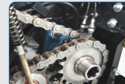
Automatic Chain Lubrication System- Longer Component Life
