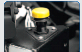
Electrical Cut Off Switch- Enhanced Safety During In Field Maintenance Activity
