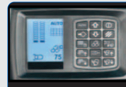
Bale Command™ Plus II Monitor (Standard) or Intelliview™ III Monitor(Optional)- In-Cab Baler control
