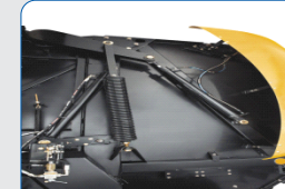
Hydraulic Density Control System- Easy Bale Density Adjustments
