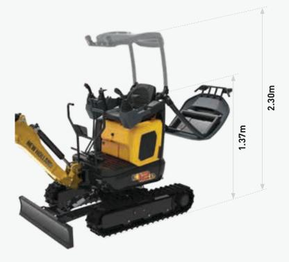
Need to access a room with low ceiling or doorway? The foldable roll-bar is easy to use, while also enabling compact machine storage without wasting building space.
