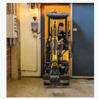
The undercarriage can easily be retracted and the blade extension folded reducing the overall machine width from 1050mm to 790mm. This enables narrow passages.
