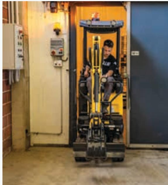
The undercarriage can easily be retracted and the blade extension folded reducing the overall machine width from 1050mm to 790mm. This enables narrow passages.
