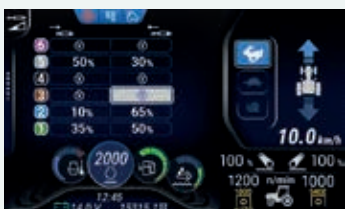
Electrohydraulic remotes flow set up
