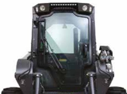
FRONT DEMOLITION DOOR
