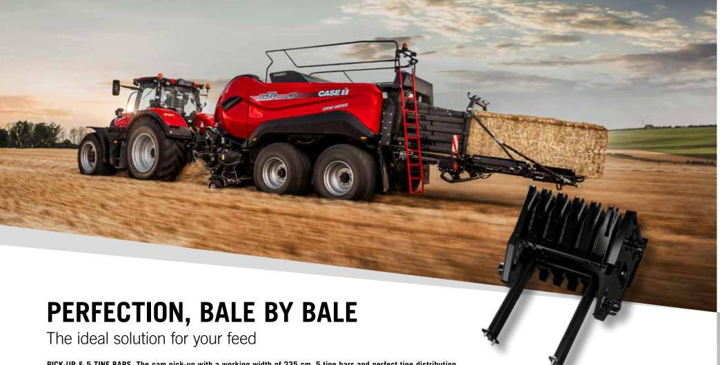
PICK-UP & 5 TINE BARS. The cam pick-up with a working width of 235 cm, 5 tine bars and perfect tine distribution reliably and cleanly picks up the swath even at higher speed.
