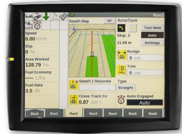
Automated turning process with AFS AccuTurn Pro
