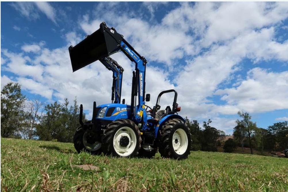
A New Holland APs30 Front End Loader system has been developed as a local, Dealer installed option. This takes advantage of the TT3.50's useful hydraulic output as well as the generous wheelbase and rated axle capacities.
