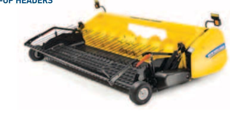
If you need to cut your crop and leave it to dry before threshing, you'll need a pick-up header. Available in 3.65 single belt and the three-belt 4.57 metre configurations, these efficient headers deliver outstanding results.
