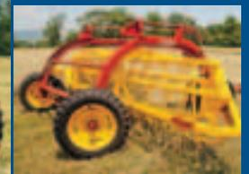
Offset wheels are set close to the basket, so the tines closely follow the ground for cleaner raking and more hay.
