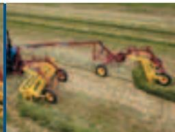
Use the Model 252 to rake two swaths into two separate windrows.
