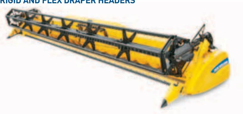
Welcome to the world of the world's largest headers, available from 6.10 to 9.15 metres cutting width. Rigid draper headers are the ideal choice when working in fields which benefit from uniform ground conditions across the entire width of the header. If you want to maintain uniform cutting performance when working in uneven terrain then the flex draper is for you.
