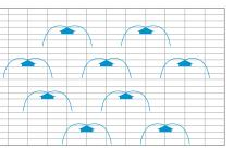
With the split-the-middle design, soil and crop residue flow equally around the sweeps for even, consistent soil and residue flow and mixing and a longer sweep lifespan.
