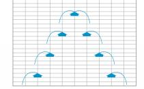
The standard V-pattern shank alignment causes uneven soil and residue flow and mixing and unbalanced sweep wear.
