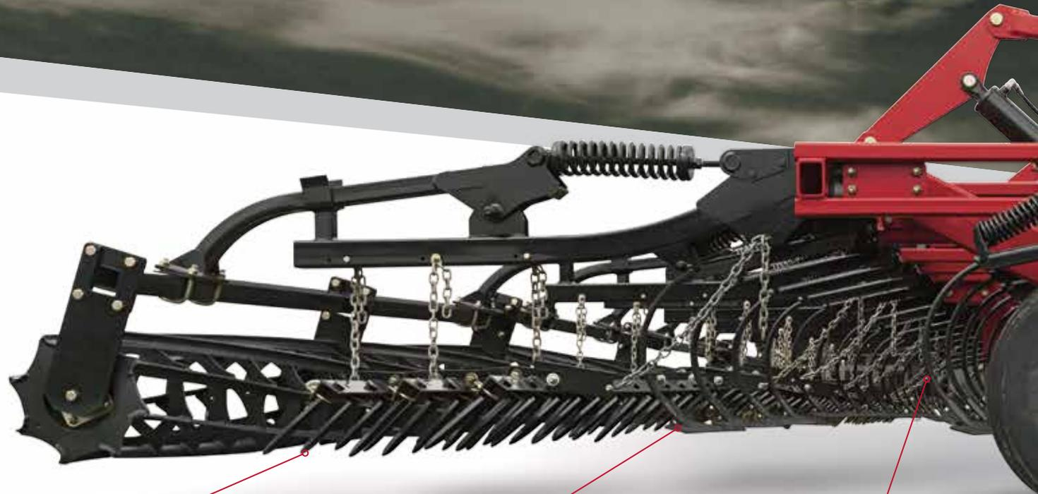
Harrow options include a **3-bar, spike-tooth** Advanced Conditioning System (ACS) harrow paired with spring or hydraulic down pressure TigerPaw™ Crumbler®. Other options include: **3-bar Extreme Tiger-Tine** ACS with Spring or Hydraulic Down Pressure TigerPaw Crumbler, **2-bar Tiger-Tine** harrow with ACS roundbar Crumbler or a **4-bar Tiger-Tine** harrow. See Page 18 for more information.
