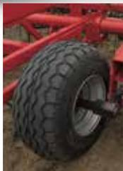
**Stubble-resistant radial tires** feature reduced compaction, improved flotation and durability in the field and during transport.
