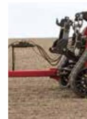
A **floating-hitch** option — available on double-fold units — allows the field cultivator to run independent of the tractor so it better follows the ground contour for improved depth consistency. *See Page 23 for more information.*
