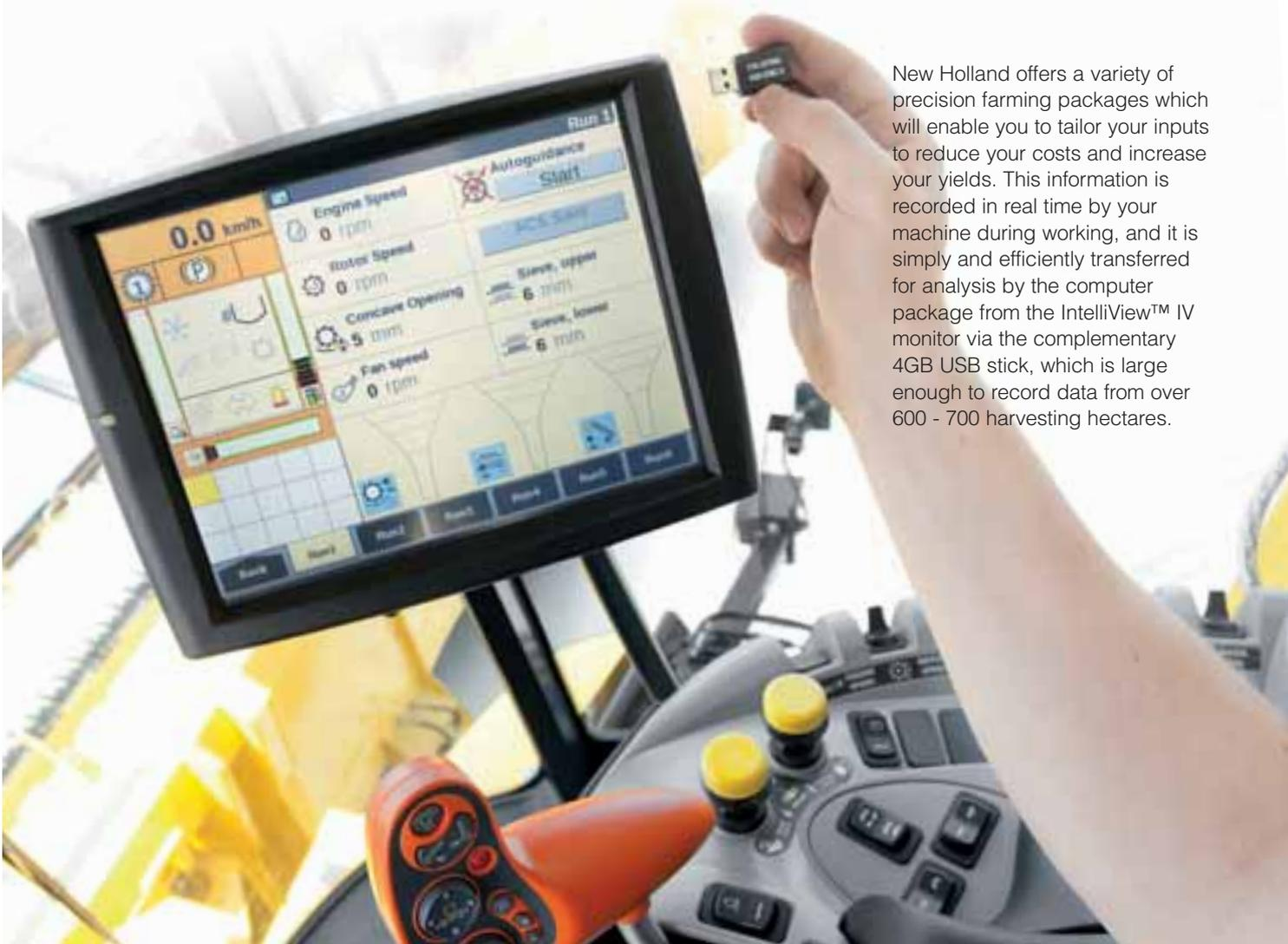
New Holland offers a variety of precision farming packages which will enable you to tailor your inputs to reduce your costs and increase your yields. This information is recorded in real time by your machine during working, and it is simply and efficiently transferred for analysis by the computer package from the IntelliView™ IV monitor via the complementary 4GB USB stick, which is large enough to record data from over 600 - 700 harvesting hectares.
