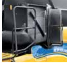
Easy access to the wide opening rotary dust screens makes cleaning the cooling package a doddle. The optional air compressor connections further facilitate cleaning.
