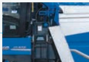
Both fuel and AdBlue tanks can be filled from the ladder for an easy access.
