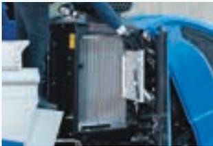
Cooling package opens out to make cleaning faster and easier.
