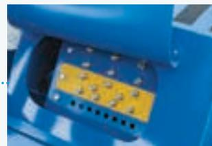
To facilitate and reduce maintenance, all harvester head grease points are grouped together and are easily accessible from the head platform.
