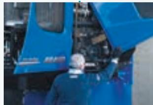
Two piece engine hood opens wide for full service access: front hood flips up perfectly for accessing engine, side door swing with a gas strut for cleaning and servicing hydraulics and coolers.
