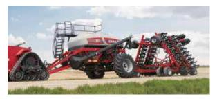
Precision Air 2355 air cart with Precision Disk™ 500 drill
