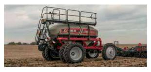
Precision Air 2355 air cart with row crop tires attached to Nutri-Tiller 955
