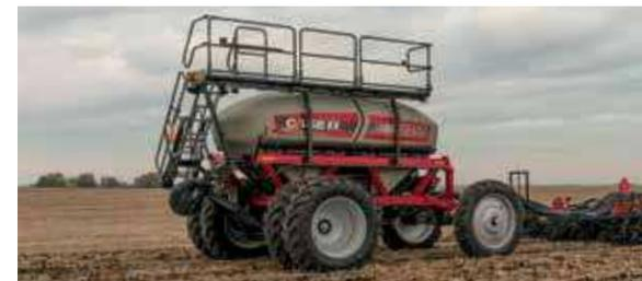
Precision Air 2355 air cart with row crop tires attached to Nutri-Tiller 955
