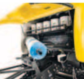
Integrated prop to support a roll of net when changing it from ground level.
