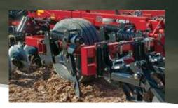
Shank depth: target the compaction layer
