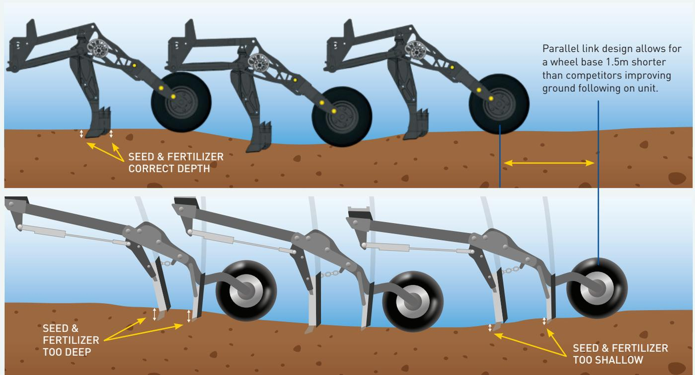
**Competitor Row Unit, Non-Parallel Link** - As opener follows terrain, seed and fertilizer depth varies (inaccuracy of placement). Machine frames have limited ground following ability (inaccuracy of placement).
