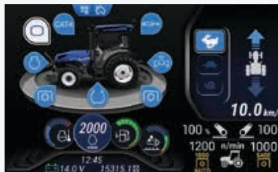
The main screen easily drive you to 8 submenu to adjust functionalities as hydraulic oil flow, PTO automatism, implement size, Blue Cab™ 4 management,... Thanks to its design and ergonomics, this screen keep the perfect visibility to outside of the cab.
