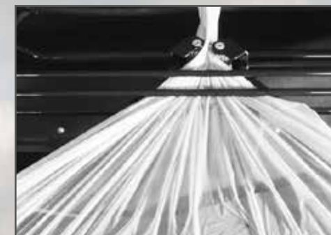
Dual pre-wrapping system with net and plastic film
