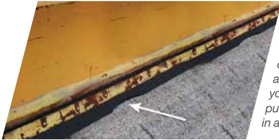
*Should a cutting edge become damaged, simply replace the section instead of replacing the entire length of a costly steel or rubber cutting edge. In the unlikely event of major damage to a section, it can be easily removed and replaced with a new replacement part from your CASE dealer. With conventional snow pushers, major damage usually results in a total loss.*
