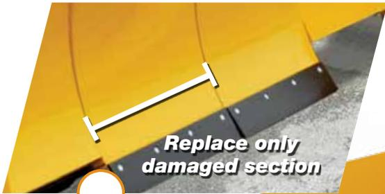
**Replace only damaged section**
