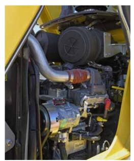
A key to equipment performance and longevity is routine care. New Holland has designed the backhoe loader so it takes the minimum of time to carry out routine checks with easy access to all key fuel, engine, transmission and hydraulic filters, and all engine servicing can be done from one sided of the machine for added convenience. Extensive New Holland's widespread dealer network will deliver expert and efficient support for your peace of mind.
