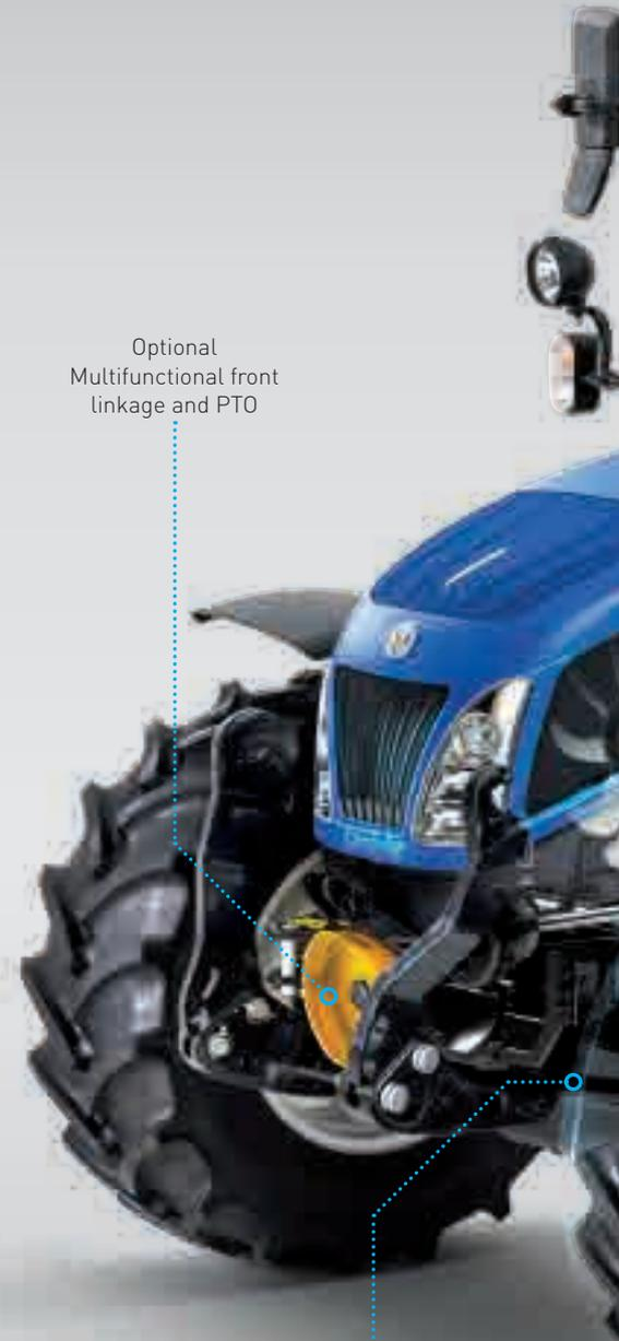
Optional Heavy Duty class 1.5 front axle allowing a gross vehicle weight of 6500kg
