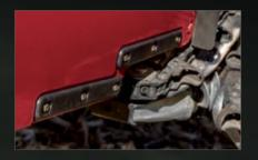
**Replaceable wear strips** are easy to service, keeping you in the field during optimal harvest windows.
