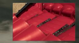
Patented CornLouvers<sup>™</sup> channel ears of corn and any loose kernels into the auger to ensure loose grain makes it into the combine.
