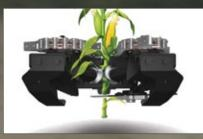
Pinching stalk rolls power feed the cornstalk directly into the path of the chopping blade and consistently deliver a 3- to 6-inch chop length.
