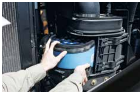
The air filter is easy to remove and the dust is aspirated and ejected in the exhaust
