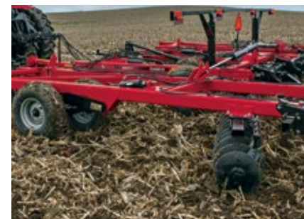
Disk gang depth: slice, cut and bury residue to the producer's desire.
