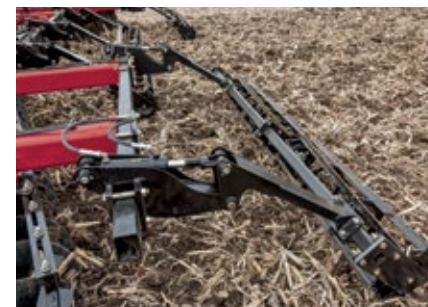
Crumbler pressure: achieve consistent clod sizing and finish.
