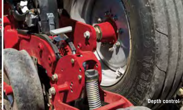
Pulled gauge wheel
