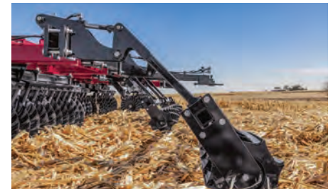
Crumbler pressure: achieve consistent clod sizing
