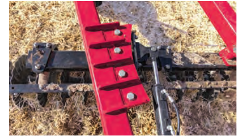
Disk gang pressure: reduce pressure on frame
