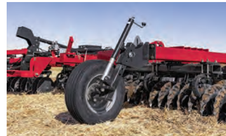
Stabilizer wheels: enhance handling and control
