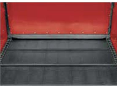
Floors are made of  $\frac{3}{4}$ " x 6" high-density polyethylene (HDPE) tongue-and-groove planks for a tight, leak-free fit.
