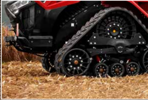
HEAVY-DUTY SUSPENSION OPTIONAL, AVAILABLE FOR ALL STEIGER QUADTRAC MODELS.
