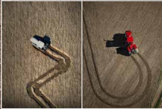
IN COMPARISON TO A 2-TRACK-SYSTEM, THE 4-TRACK-SYSTEM STEERS UNDER FULL LOADS, MINIMISING SOIL DISTURBANCE WHEN TURNING.
