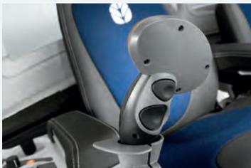
Shift button and ground speed unlock (behind).
