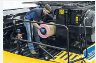
The air filter is easily accessible from the engine platform.
