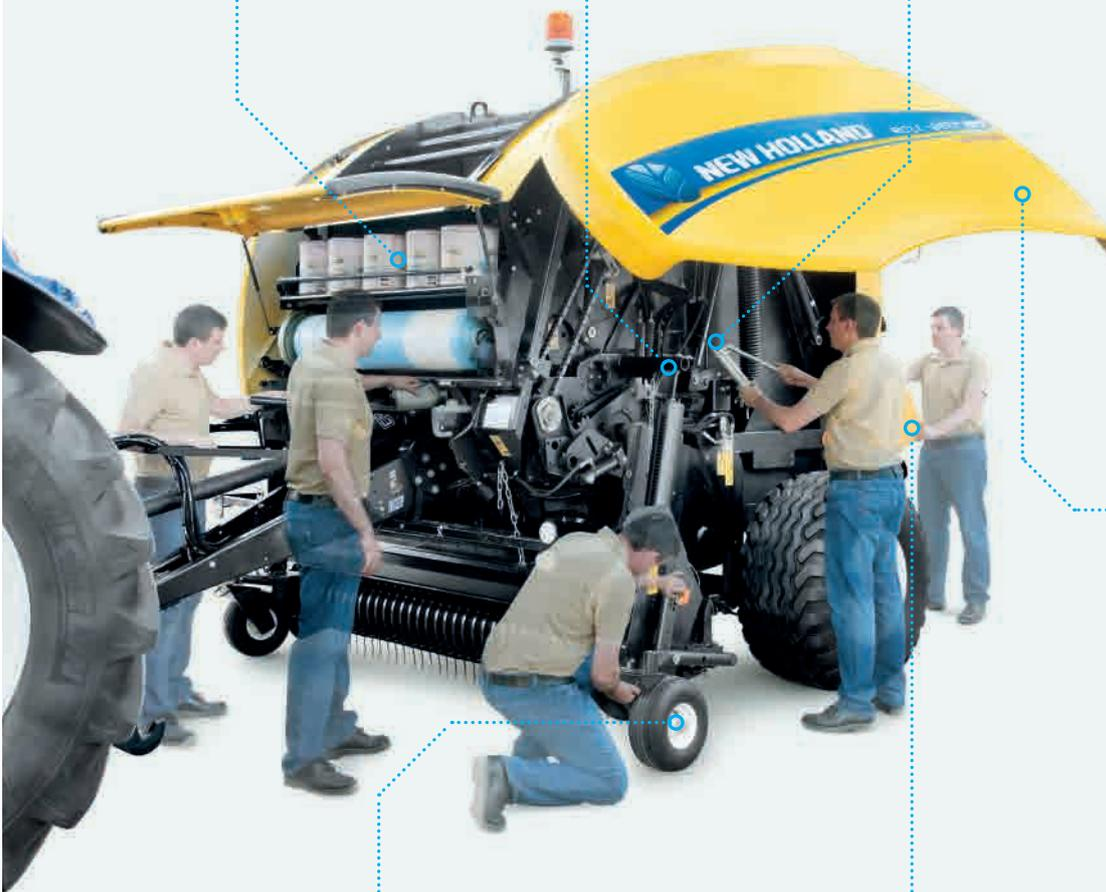
Pick-up wheels switch from field to transport mode without the use of tools.
