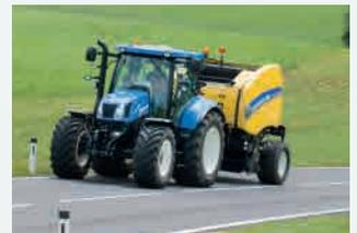
Optional ultra-wide 500/55-R20 tyres reduce compaction to facilitate regrowth for subsequent silage cuts. They also deliver more comfortable road transport.
