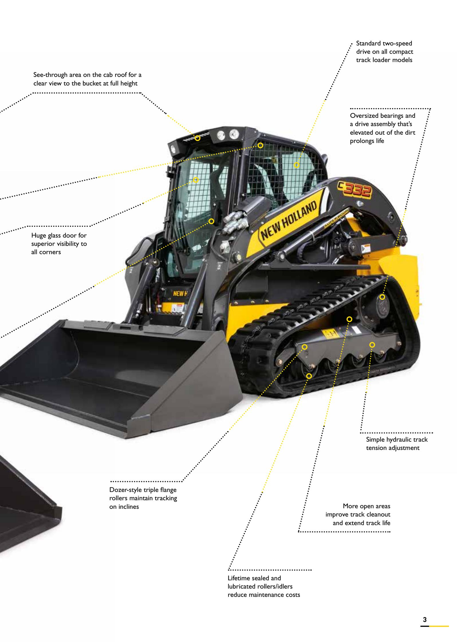
Standard two-speed drive on all compact track loader models
