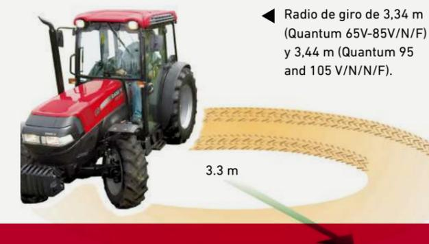
◀ Radio de giro de 3,34 m (Quantum 65V-85V/N/F) y 3,44 m (Quantum 95 and 105 V/N/N/F).
