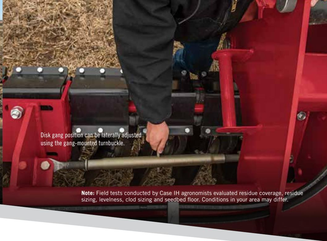
Disk gang position can be laterally adjusted using the gang-mounted turnbuckle.
