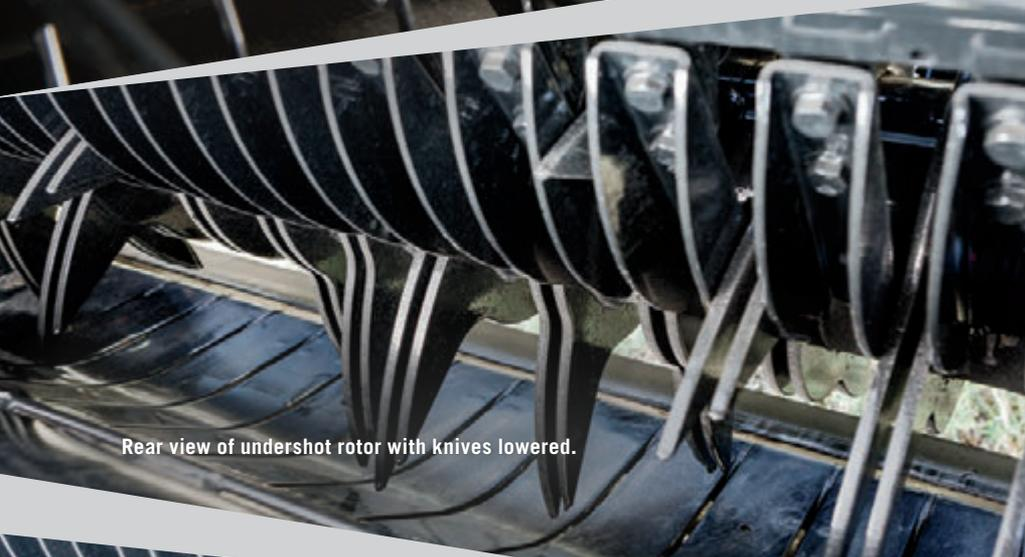
Rear view of undershot rotor with knives lowered.
