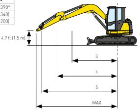
The lifting capacity is based on the ISO 10567 and it does not exceed more than the 75% of static tipping load or more than the 87% of the hydraulic lifting capacity of the machine.
