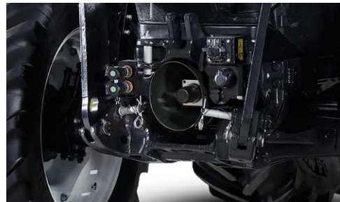
New front PTO design with wet clutch
