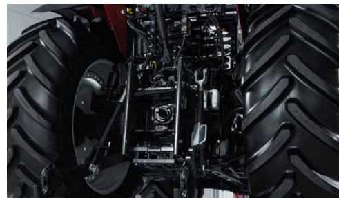
Rear lift capacity 4,700 kg
