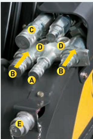
A connect under pressure CUP hydraulic manifold is standard equipment on all models for easy hook-up of all hydraulic attachments. By pushing on the fitting, you release pressure in both hydraulic lines.
