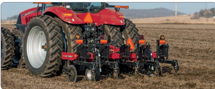
Case IH Ecolo-Til® 2500 disk rippers can be customized to leave the soil and residue visually undisturbed. They provide a soil/residue mixture that allows rain to soak down into the subsoil faster, decreasing erosion through improved porosity and drainage.
