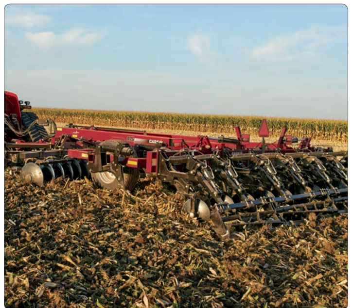
Combination primary tillage tools, like the Ecolo-Tiger 875, can manage crop residue, soil tillth and provide a level seed bed in a single pass.
