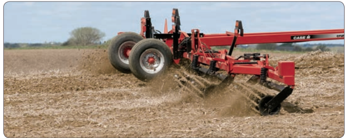
The attachable Case IH Crumbler® seed bed finisher combines primary tillage tools or the Tiger-Mate 200 field cultivator with secondary tillage in one pass. It provides the final touch for thorough seed bed preparation by creating an excellent seed bed of firm, fine soil covered by loose, coarse soil.
