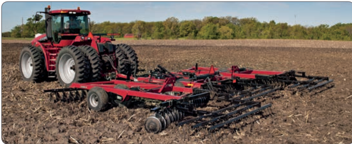
Case IH True-Tandem™ 340 and 370 disk harrows are high-performance seed bed preparation systems that help properly distribute residue, size clods and firm the seed zone to achieve the desired field finish.
