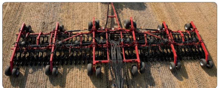
The Precision Disk™ family of air drills feature a parallel-link system, consisting of an upper and lower arm to ensure even depth placement across varying soil conditions. Patent-pending variable down-pressure springs apply the right amount of pressure on individual row units to ensure better penetration across varying residue and soil conditions.
