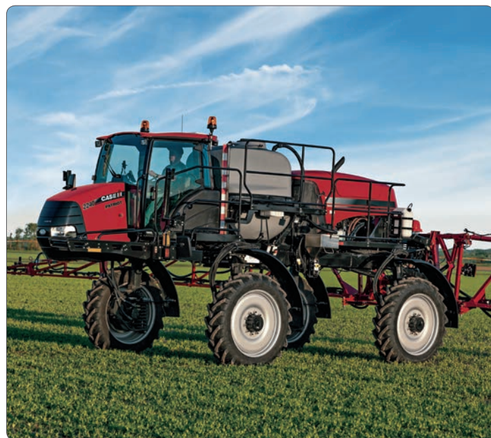
Case IH equipment, like this Patriot 4430 sprayer, is designed to deliver even weight distribution, which means less rutting and soil compaction in wet conditions.
