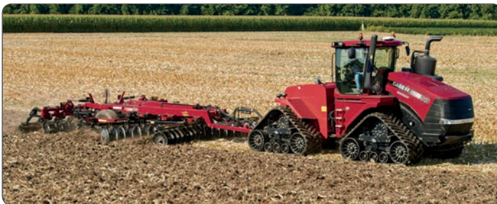
Case IH Ecolo-Tiger® 875 disk rippers offer all-new redesigned, high-density Tiger Points that run just under hardpan compaction and deliver the proven Case IH lift-twist-roll soil action to eliminate soil compaction, but with less draft. This contributes to smoother fields and extended point life.
