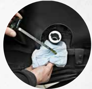
Oil level check and top up without lifting the bonnet
