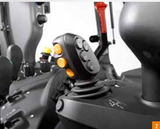
1 Joystick for front loader work on the PROFI, PROFI CVT and CVT
