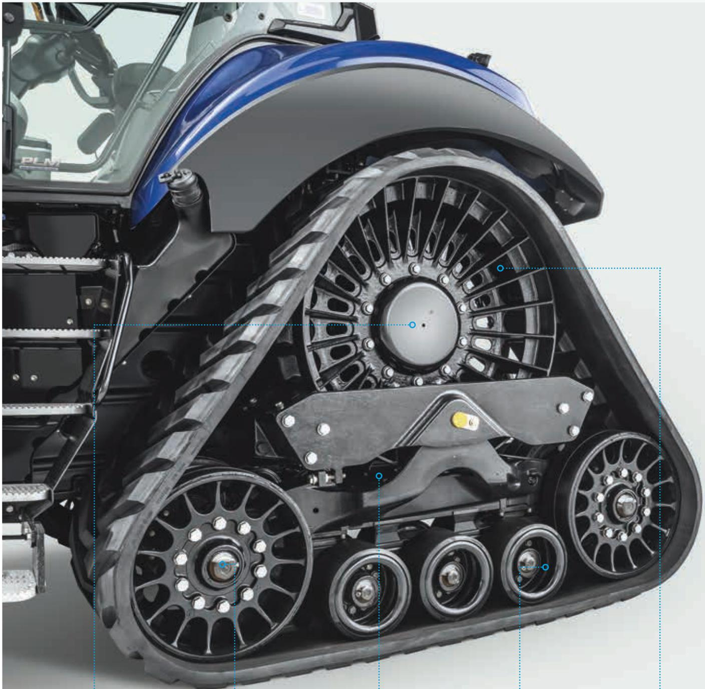
Ductile cast iron drive wheel
