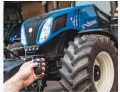
**Factory installed remote locking and immobiliser**
