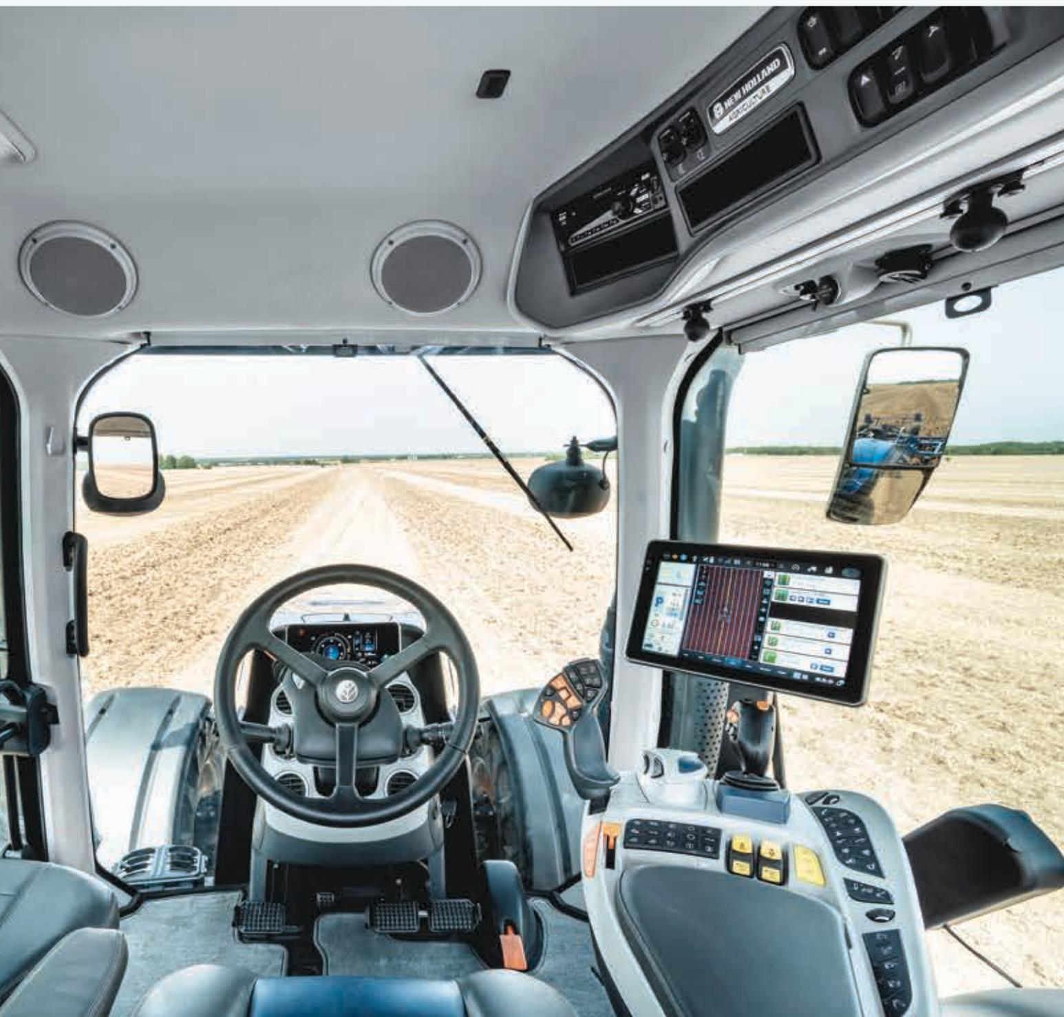
Thanks to a laminated front windscreen, thicker rubber window and door seals, thicker floor mat and even more insulation under the cab floor, the new T8 Genesis™ cab is even quieter than ever.
