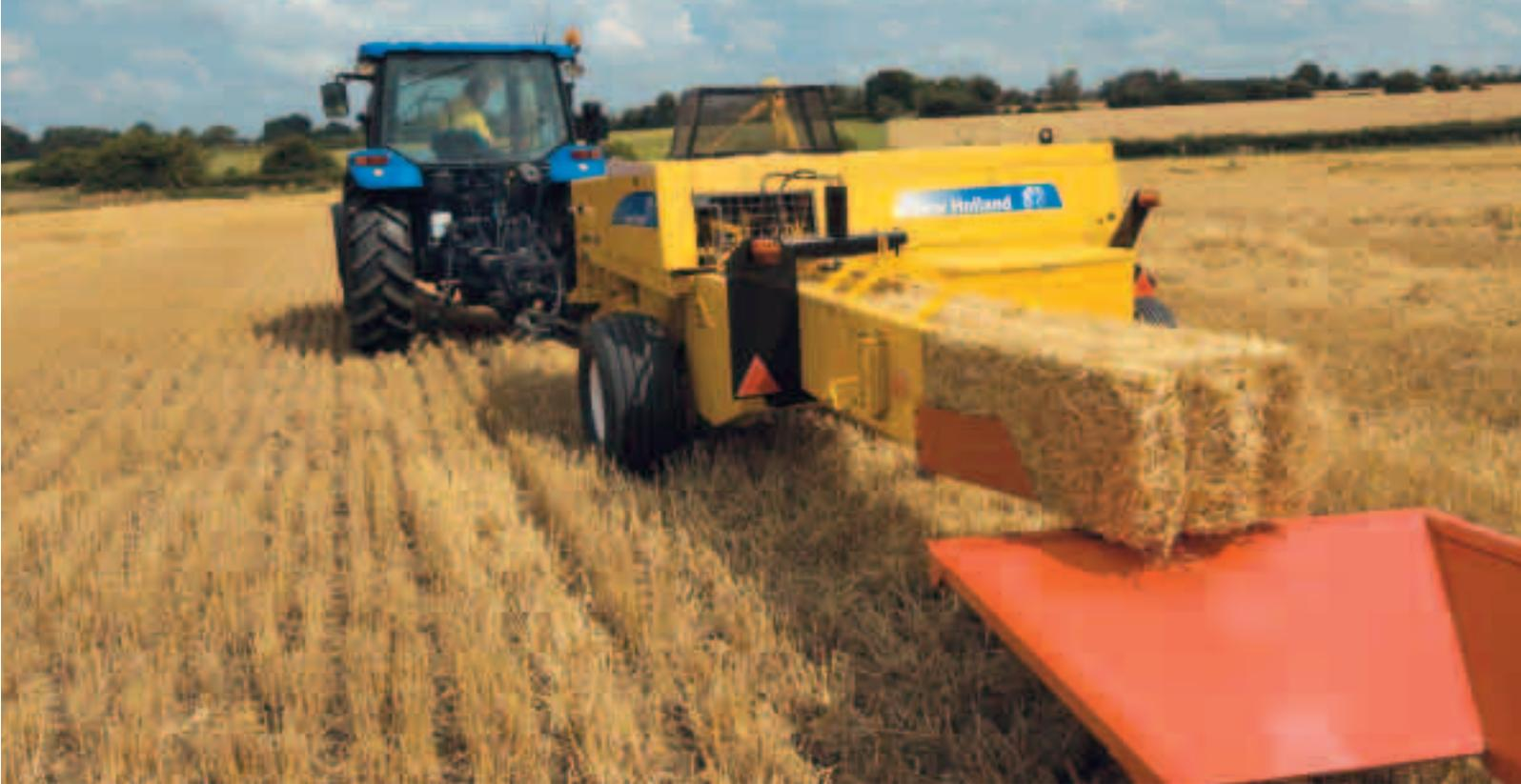
Producing consistent firm bales is a major benefit of the new BC5000 balers. The long bale chamber, allowing for a long plunger stroke, combined with the high plunger speed, ensures a 1st class quality bale formation. Adjustable top and bottom bale chamber rails and adjustable bale case doors allow for a perfect setting of the required density.
