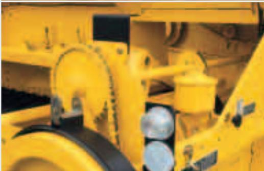
Producing high quality bales day after day, season after season requires robust and reliable drive lines. The dimensions of the shafts, chains and gears as well as the quality of the steel, reflect New Holland craftsmanship and experience. To prevent the build-up of stress on the functional components, the overall baler construction includes a draw bar that is directly connected to the baler axle. A “power pivot support” for the three-joint PTO furthermore allows sharp turns with maximum safety.
