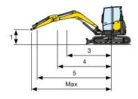
The lifting capacity is based on the ISO 10567 and it does not exceed more than the 75% of static tipping load or more than the 87% of the hydraulic lifting capacity of the machine.
