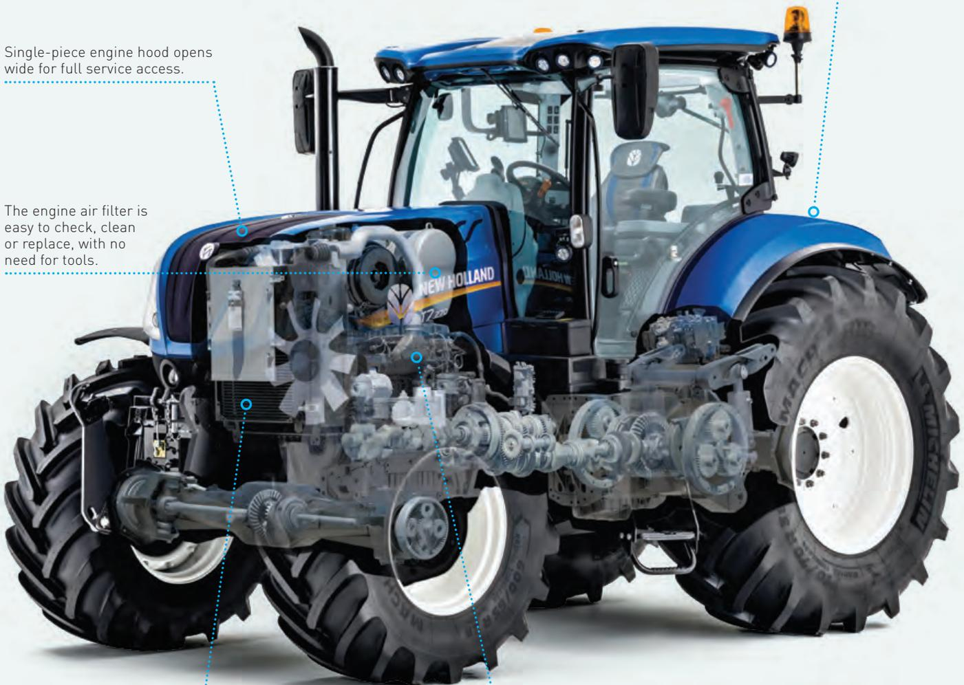
Cooling package opens out to make cleaning faster and easier.
