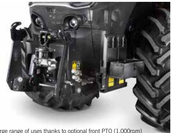
Large range of uses thanks to optional front PTO (1,000rpm)
