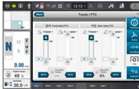
Intuitive layout for the automatic on/off settings for the height-dependent front and rear PTO
