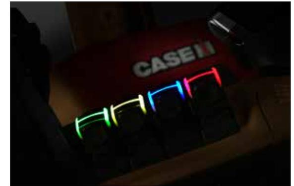
Configurable control switches with changing colours enable the individual assignment of the rear control units in the armrest.
