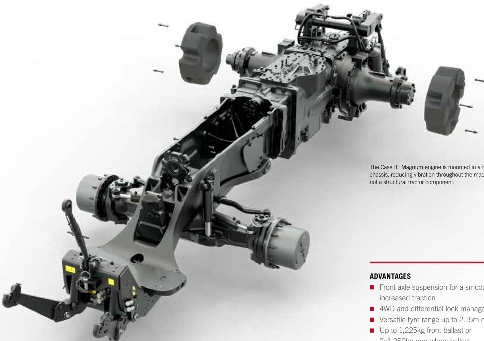
The Case IH Magnum engine is mounted in a heavy cast contoured chassis, reducing vibration throughout the machine as the engine is not a structural tractor component.
