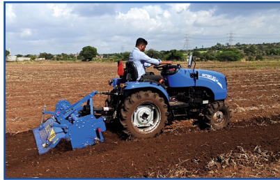
Rotavator Gear ERPM PTO RPM L1/L2 2600 540
