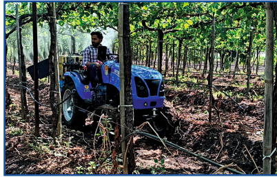
Electrostatic Sprayer Gear ERPM PTO RPM L2/M1 2600 540
