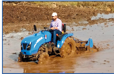
Puddling Gear ERPM PTO RPM L2 2600 540
