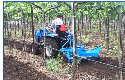
Ridger Gear ERPM H1 1400-1600
